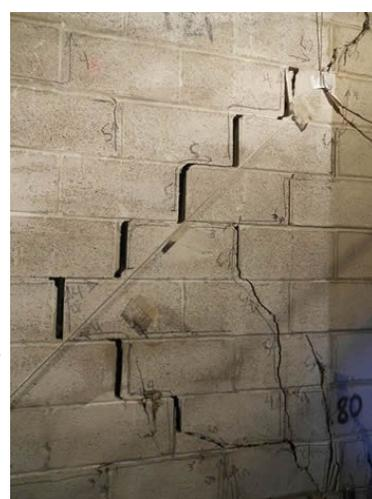
Damage after destructive testing
